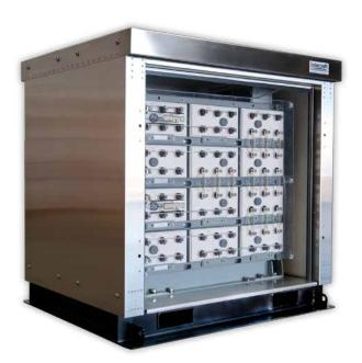
Front and back removable bolt-on doors provide access to both sides of the enclosure, and allow flexibility in site layout. Memory-resistant door gaskets create a water tight seal. Passive ventilation for battery gas is accomplished with recessed vents at the top and bottom of the enclosure.
